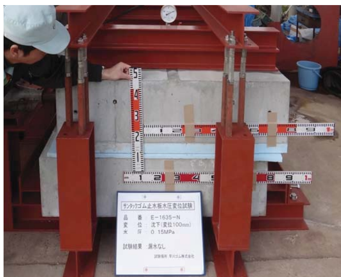
沈下量100mm/耐水圧0.15MPa
