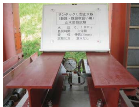
伸び量30mm/耐水圧0.1MPa
