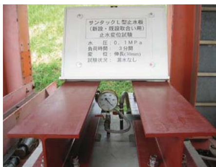
伸び量30mm/耐水圧0.1MPa
