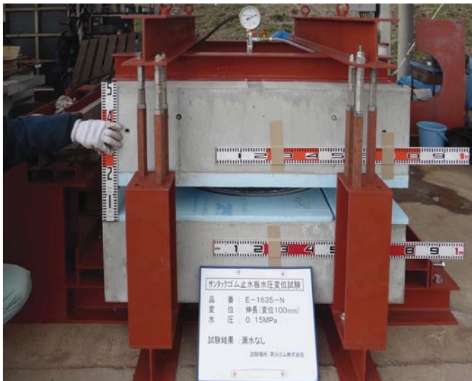
伸び量100mm/耐水圧0.15MPa
