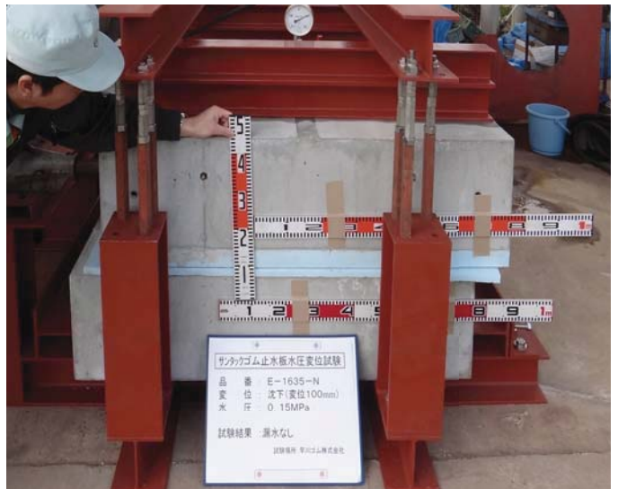
沈下量100mm/耐水圧0.15MPa
